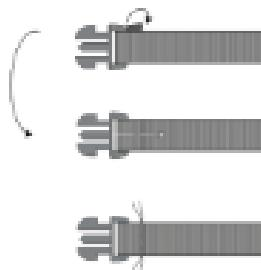
**STEP 7:** To make the right side of the waistband, feed the 31 "(78 cm) long webbing through the two slider holes and secure the webbing with a straight seam.
