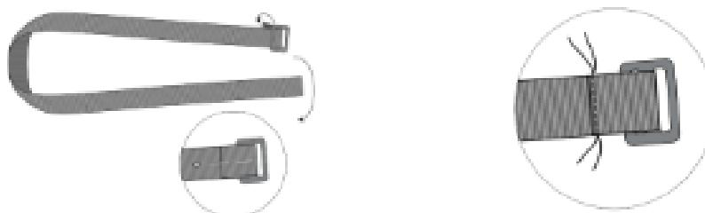
**STEP 8:** Then insert the tape through the two holes on the female side of the buckle, pass the tape through the slider again.
