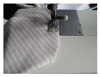
Sew the two remaining sides as well, make sure that you always sew to the end point of the first seam.
